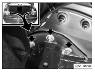
Loosen left/right inner nuts and adjust height of bumper. For tightening torque, refer to Technical Data 51 12 2AZ
